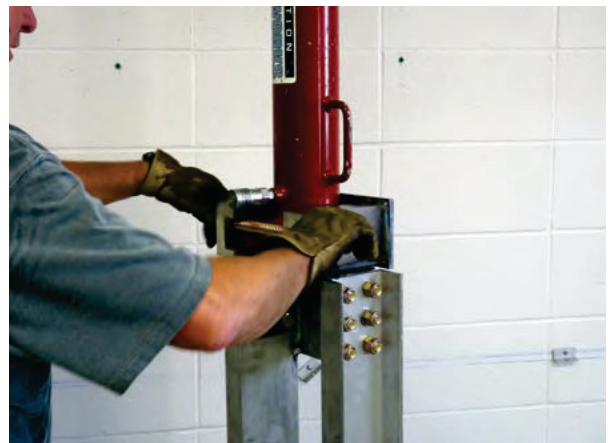
Figure 2.73 Drive cylinder set into top fixture of drive stand
